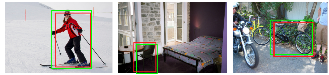
Figure 4: Examples of noisy bounding boxes generated by the jittering procedure used to prepare training data for Snapper’s adjustment model. Unaltered ground truth boxes are shown in green while jittered boxes are in shown in red.
